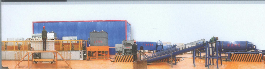
Rotary rolling grinding ball automatic production line, originated by Huamin. Equipment Patent Number: ZL200610043960.1
