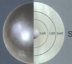
Sectional view for measuring points in a steel ball
